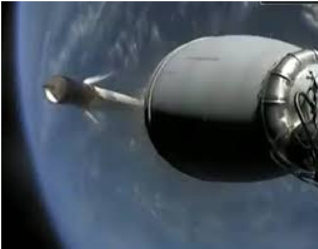
Figure 1: Falcon 9's cold gas thrusters firing to reorient the first stage
