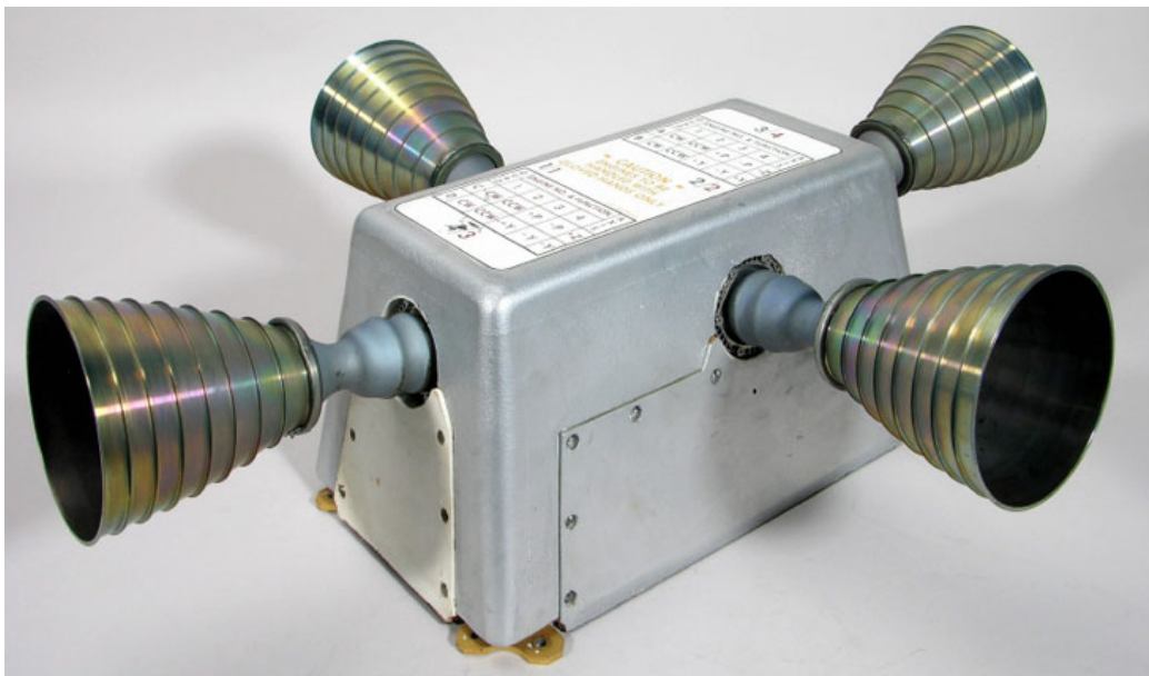
Figure 2: An Apollo service module RCS thruster block
