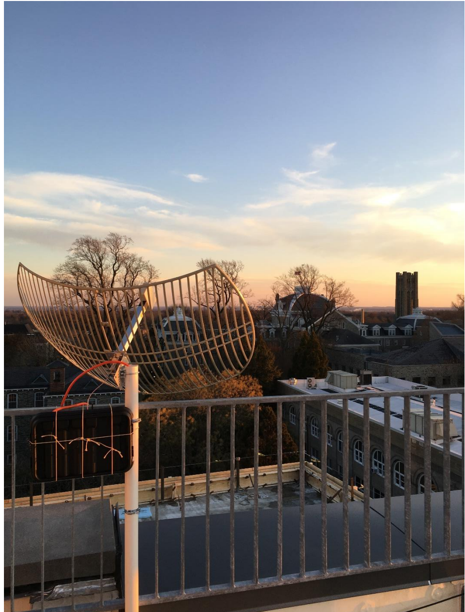
Figure 2: Suggested Receiver Station Setup with a 1.7 GHz grid dish antenna mounted on a PVC pipe. Electronics are housed in a strapped-down waterproof box with conduits for the RF cable and extension cord.
