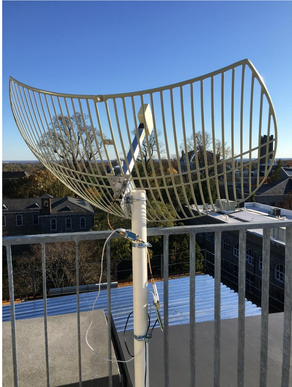
Figure 3: A picture of the receiving station that shows the electronics components. Starting from the antenna, the line in uses an N-type to SMA adapter, a 6in shielded SMA cable, a Nooelec SAWbird+ GOES filter (powered by the Raspberry Pi via microUSB wire), another 6in shielded SMA cable, Airspy Mini SDR device, and finally, a Raspberry Pi 3B+.
